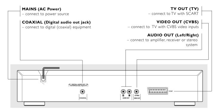
Caution: Do not touch the inner pins of the jacks on the rear panel connectors. Electrostatic discharge may cause permanent damage to the unit.
